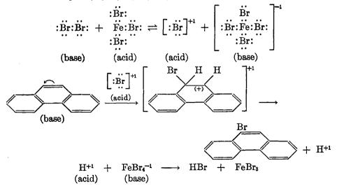
Other acidic compounds such as antimony pentachloride, stannic chloride, and iodine can catalyze the reaction through the hetero-fission of the bromine molecule and the formation of the polar complex.
