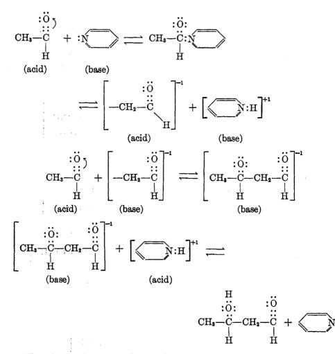
When the reaction is carried out in deuterium water (9) no deuterium hydrogen becomes attached to the carbon, indicating that water takes no direct part in the mechanism of the reaction.
