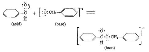
A second molecule of aldehyde reacts as an acid with this intermediate and removes a hydride ion, thus forming the neutral ester molecule and at the same time regenerating the basic catalyst, i.e., the benzylate ion:
